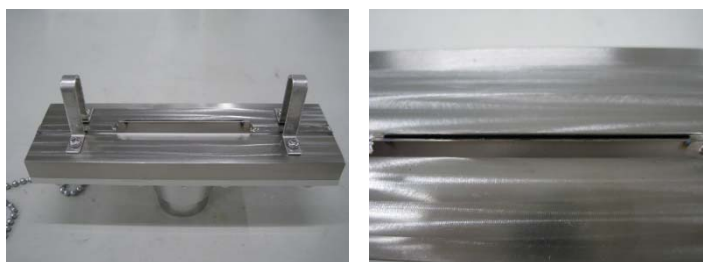
Figure 4 - High-temperature burner (left) and close-up of flame outlet after completion of measurements (right)
